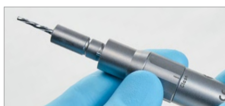
Close the fixing ring of the craniotome's handpiece. The drill now resists being pulled out.
