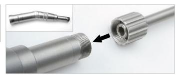
Insert the burr shank into the open collet chuck of the angled handpiece as far as it will go and close the collet chuck by turning the clamping sleeve.
