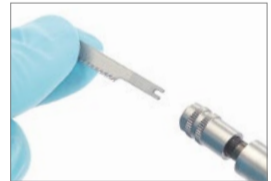
Remove the saw blade from the collet and replace if necessary.
