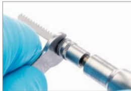
Loosen fastening nut with hook spanner
