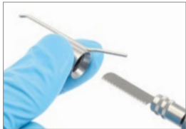
Remove the cooling clip from the saw handpiece.
